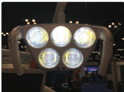
Figure 2 LED array on modern operating light (5 lites on 1 fixture).
