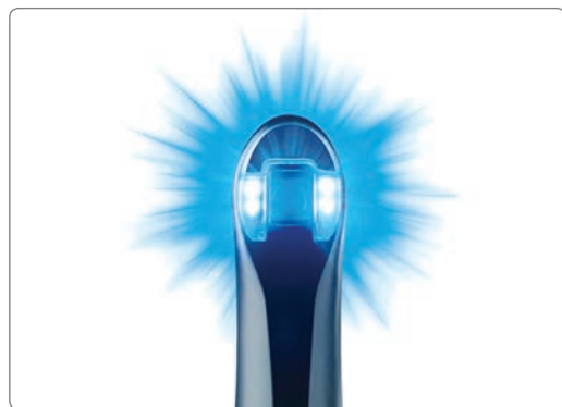
Figure 5 The blue fluorescence mode is also included in the head of the camera where four blue LEDs emitting at a wavelength of 450 nm are located.
