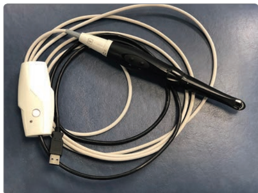
Figure 2 SoproLife cable. Connection to the handpiece at one end and the USB connector at the other end of the cable.
