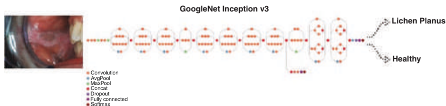
Fig. 9.8 An artificial intelligence model was developed using TensorFlow Inception V 3 architecture, which is a deep learning approach. Figure shows the whole procedure for identifying skin disease using deep learning-based techniques. The intraoral photos are entered into the system and processed in this manner. To evaluate if the disease is present, the input image is analyzed using image processing techniques such as preprocessing, feature extraction, and a machine learning-based classifier. (Reproduced from Keser et al. 2023)
