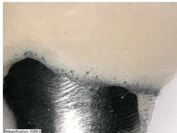
Figure 7.35 Ceramic layer porosity. Usually seen overlapping the abutment margin and extending to the gingival area.
