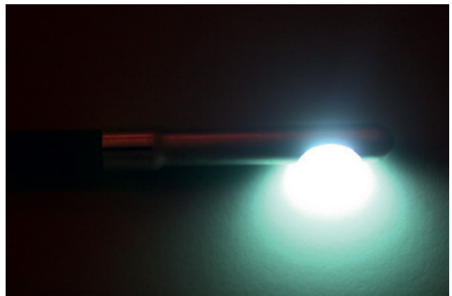
Figure 27.12 (a) Prototype UVC handpiece with mercury ray tube. (b) Gated shield directing the UVC energy to the target tissue.
