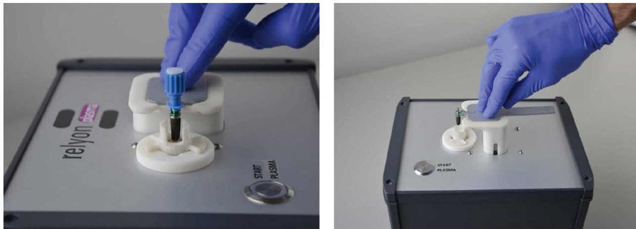
Figure 29.6 Images of a user placing an implant into the implaPrep concept device. Source: Courtesy of RELYON PLASMA GMBH.
