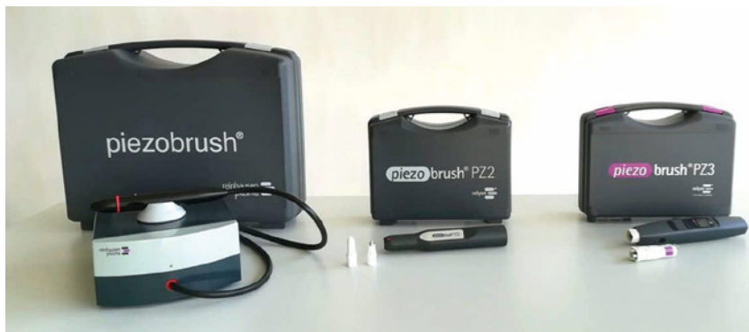
Figure 29.9 Three generations of the piezoelectric direct discharge based piezo brushes. Source: Adapted from Korzec et al. [46].
