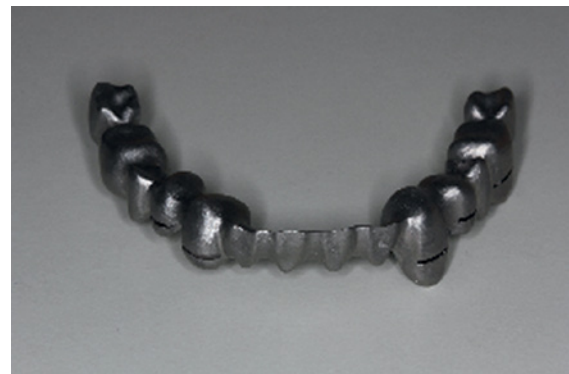
Workflow: figures 13 and 14: Tertiary framework designed by CAD and milled by CAM.
