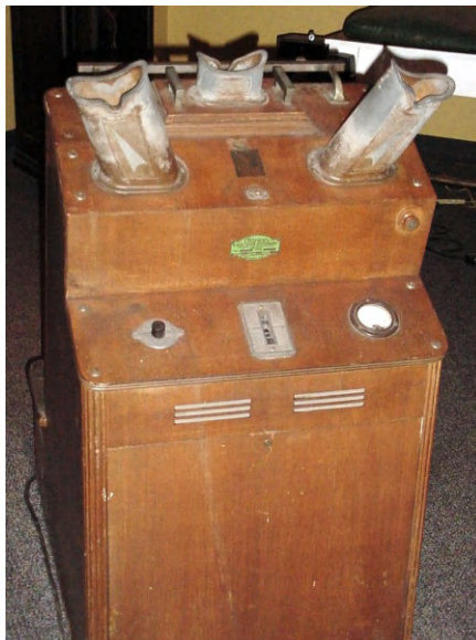
Figure 87. A shoe fluoroscope. (Image obtained from Wikimedia Commons, the free media repository)
