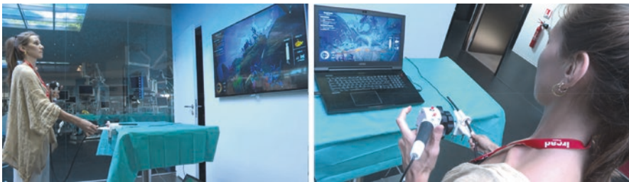
Fig. 3.2 Overview of the endoscopic serious game rescue in the deep. Students can be trained in a friendly sea environment. Five training levels that allow navigation, targeting, and coordination are considered
