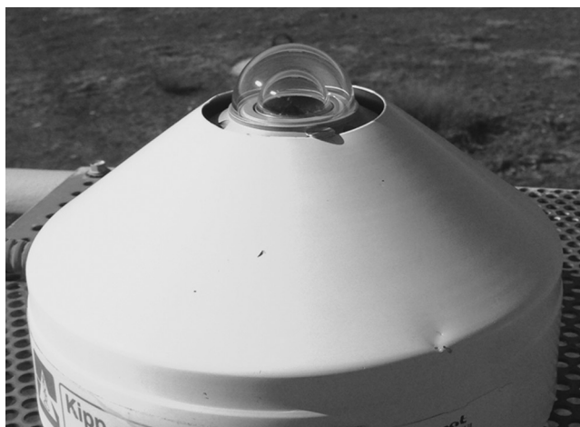
Figure 9.1 Pyranometer and its sun shield.
