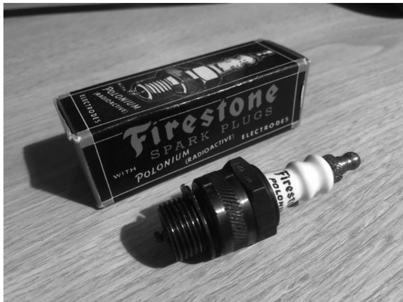
FIGURE 12.7 The Polonium Spark Plug produced by the Firestone Tyre and Rubber Company.
