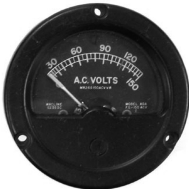
FIGURE 5.4 Luminescent voltmeter gauge.
