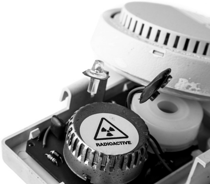
FIGURE 10.1 Location of the americium-241 source in a domestic smoke detector.
