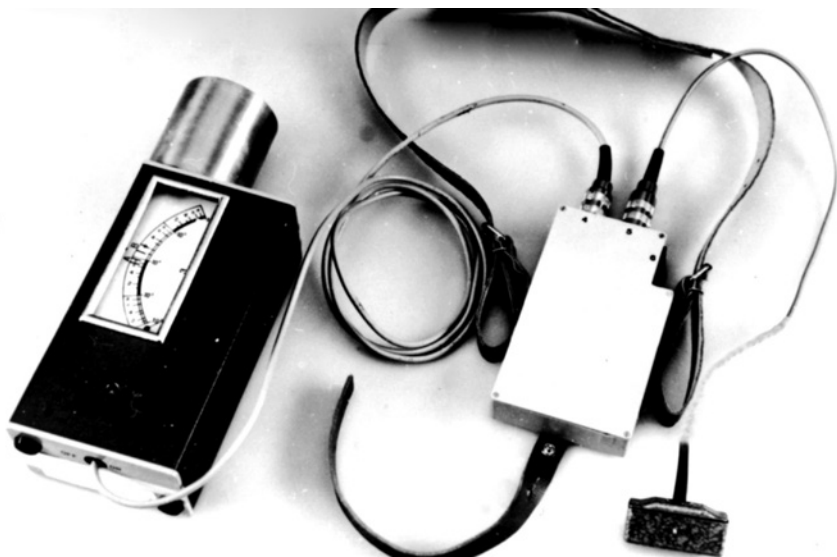
FIGURE 12.2 The Cloud 005 scintillation detection instrument on the left was powered by a battery pack. The small black vibrator pad worn near the skin of the agent can be seen on the bottom right.
