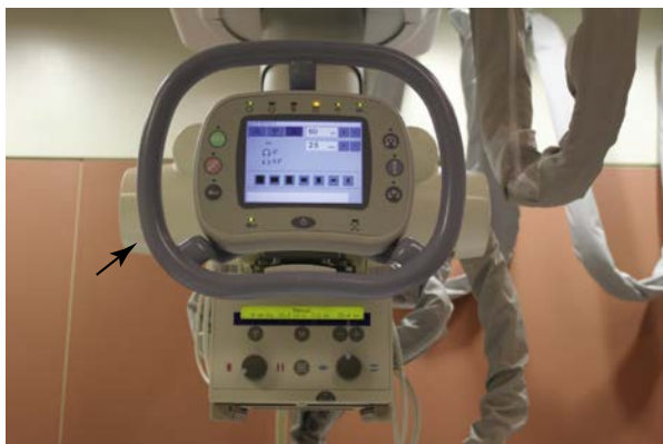
Fig. 1.15 The tube housing ( arrow ) shields the tube and provides mounting for tube motion controls and collimator.
