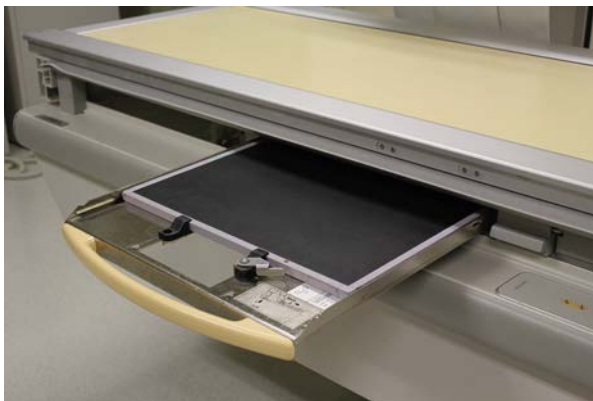
Fig. 1.22 The bucky tray holds the image receptor within the x-ray table.
