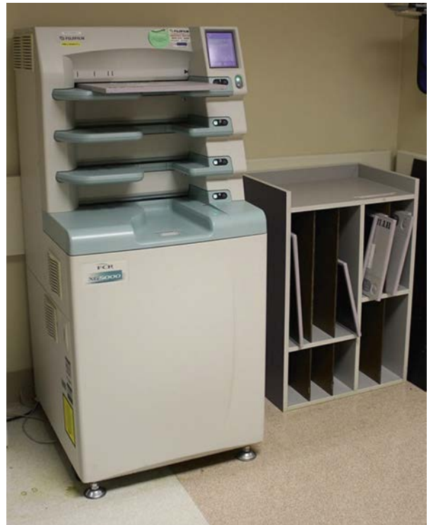
Fig. 2.3 Image processor for a computed radiography system. Note the computed radiography cassette storage system to the right of the image processor.
