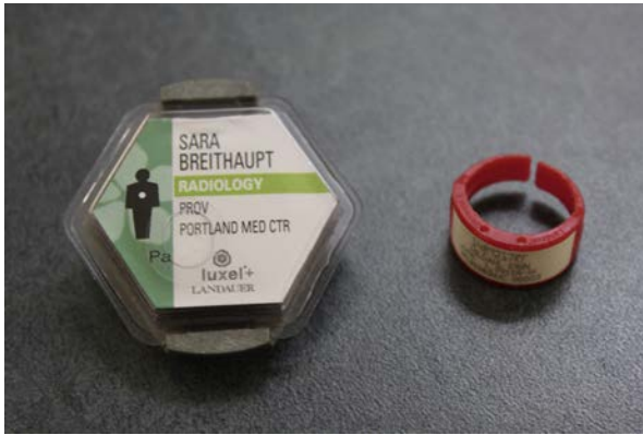
Fig. 3.2 Left: The current generation of personal dosimeters is the optically stimulated luminescence type. Right: Ring badge for workers whose hands receive more than their total body radiation exposure, such as those who handle radioactive materials.
