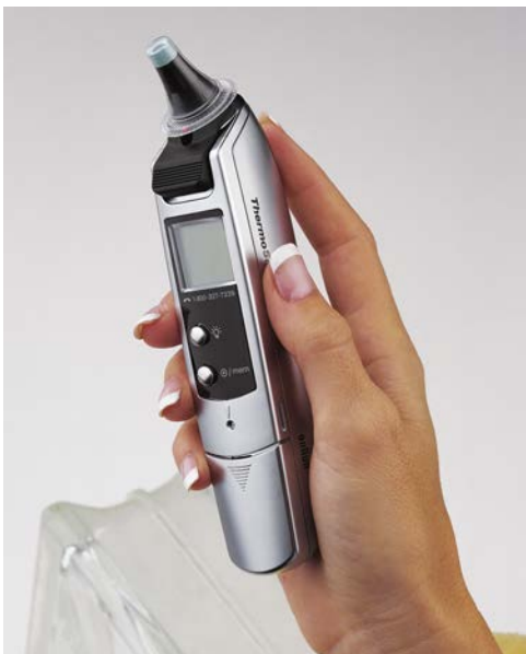
Fig. 13.3 Tympanic thermometer probe is inserted into external auditory canal. (Courtesy Welch Allyn; Skaneateles Falls, NY.)
