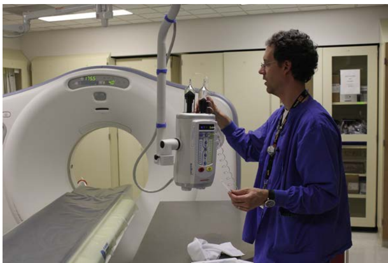
Fig. 22.21 Automatic injector controls administration of contrast for computed tomography examinations.
