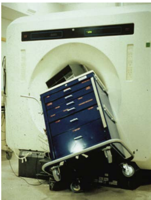
Fig. 22.30 A metal emergency cart lodged within the gantry of the magnetic resonance imaging (MRI) machine. Common medical equipment can quickly become projectile objects that lodge in the center of an MRI machine. (From Coté CJ, Lerman J, Todres ID: A practice of anesthesia for infants and children , ed 5, Philadelphia, 2013, Saunders Elsevier.)
