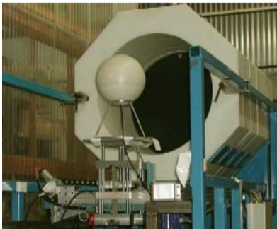
FIG. 2.VII.1 – (left side) Picture of the CANEL/T400 facility with a single Bonner sphere, (right side) layout of the CANEL apparatus as modeled in MCNP (from Lacoste et al. , 2011).
