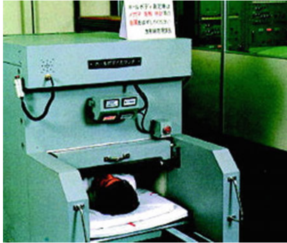
Fig. 6.7 A whole-body counter for determination of profiles of EQ in a human body
