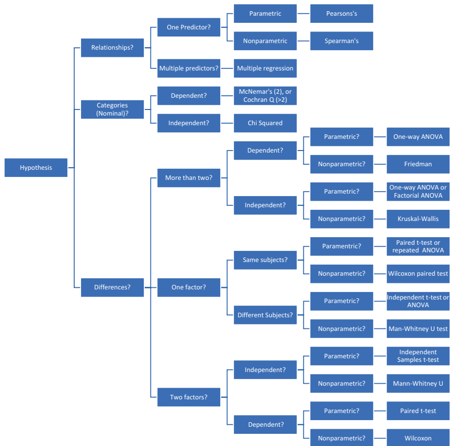
Fig. 6.13 A decision tree for statistical tests based on a combination of guidance given by Field A. (2013). Discovering statistics using IBM SPSS statistics . Sage and Pirk, C. W., et al. (2013). Statistical guidelines for Apis mellifera research. Journal of Apicultural Research , 52(4), 1–24 and (Neill Howell 2008 Inferential Statistical Decision Tree - StuDocu, n.d.)
