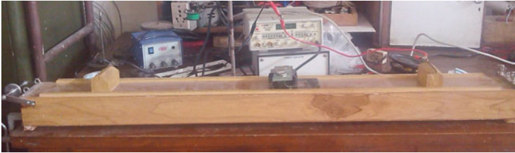
Fig. 3 Wire tension measurement setup at Panjab University
