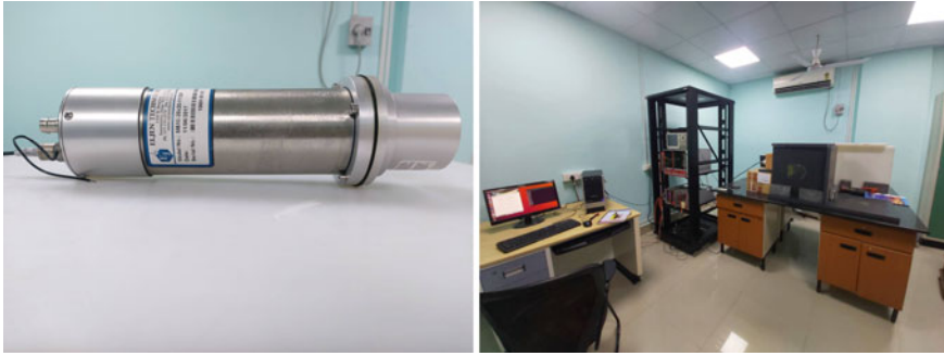
Fig. 1 (left) EJ-301 detector coupled to a photo-multiplier tube. (right) Complete experimental setup consists of detector, power supply, digitizer, shielding, radioactive sources and PC
