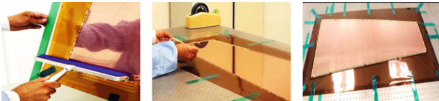
Fig. 3 Cleaning of the GEM Foils (Left), Placing the spacers (Middle) and Assembled GEM stack (Right)
