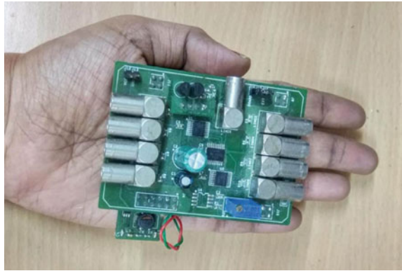
Fig. 1 C-DAQ compact data acquisition module
