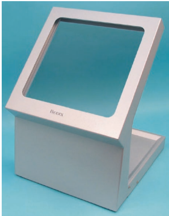
Fig. 4.2 Tabletop L-Block shield (for beta and gamma radiation) (photo courtesy of Capintec)
