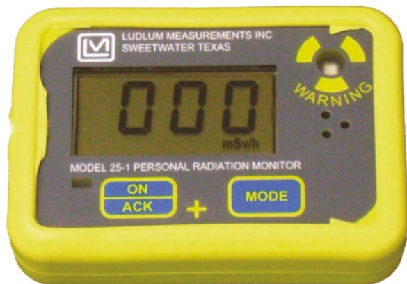
Fig. 2.21 Electronic personal radiation monitor M25-1 (courtesy of Ludlum instruments Inc.)
