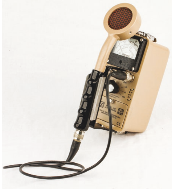
Fig. 2.11 A Ludlum G-M survey meter with a pancake probe (courtesy of Ludlum/Pinestar technology)
