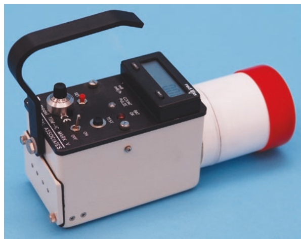
Fig. 2.3 A digital cutie pie survey meter (photo courtesy of Capintec)
