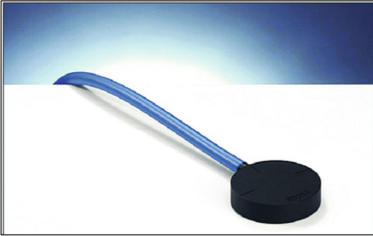
Fig. 11 Plane parallel ionization chamber for reference high-energy electron dosimetry [16]
