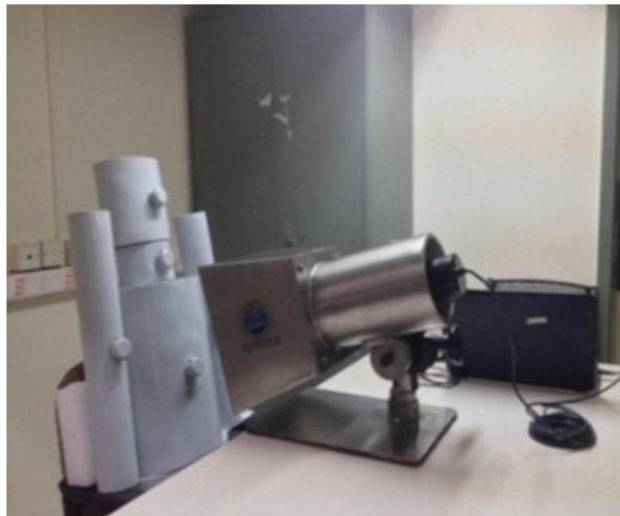
Fig. 4 Portable thyroid monitoring system along with a typical ^{131}\text{I} spectrum and IAEA/ANSI neck phantom
