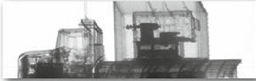
Fig. 10 Gamma-ray image of a truck showing goods inside a shipping container [25]
