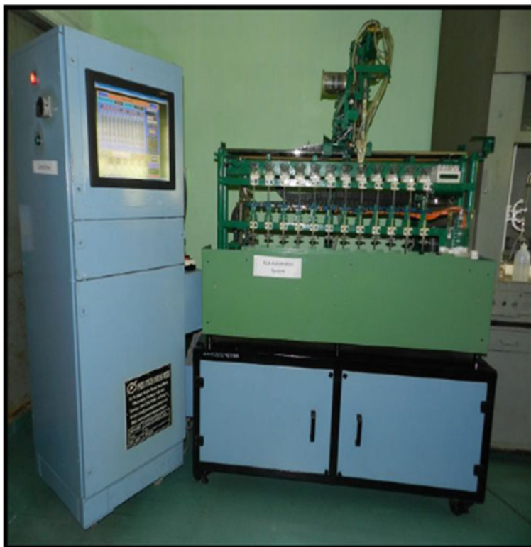
Fig. 15 Photo of automation system for radiochemical separation of actinides based on ion-exchange
