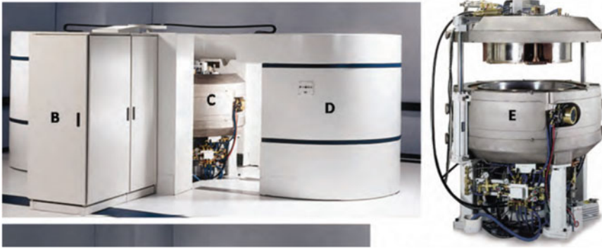
Fig. 18 Commercial self-shielded cyclotron for radionuclide production. Proton beam energy of 11 MeV and beam current 60 \mu\text{A} . B: Power supply and control cabinet, C: Cyclotron assembly, D: Retractable radiation shielding and E: Cyclotron assembly
