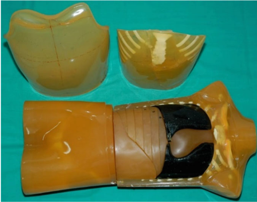
Fig. 16 JAERI Phantom with lungs, heart, and chest overlay with rib bones
