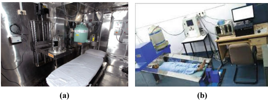
Fig. 5 (a) HPGe array for lung monitoring of actinides and (b) HPGe detector in scanning WBC
