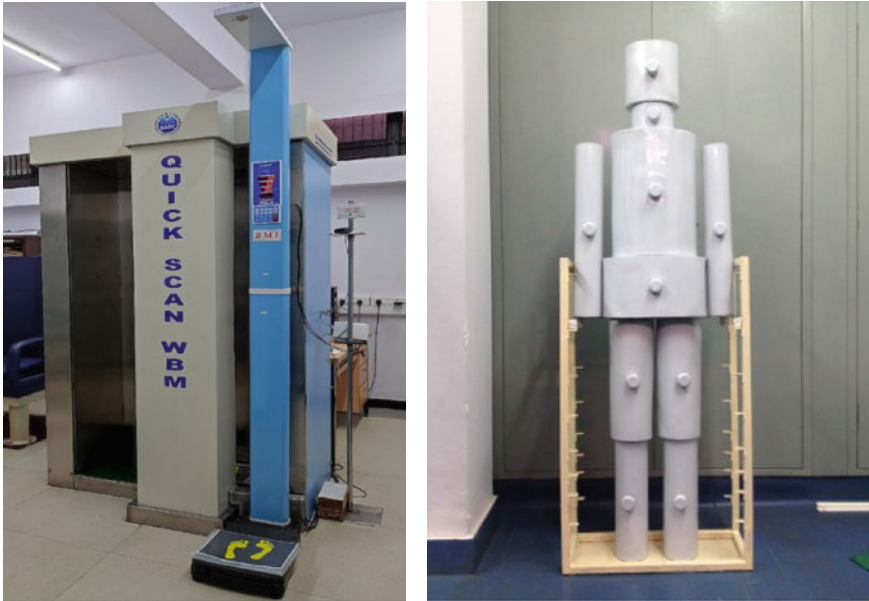
Fig. 6 Standing type whole body monitor for rapid screening of individuals for in-vivo monitoring of high energy gamma emitters and BOMAB phantom
