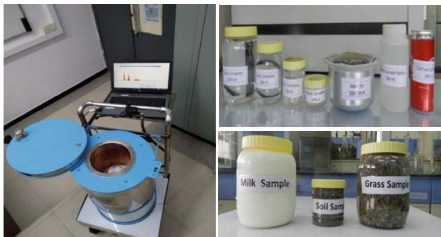
Fig. 7 Vehicle mountable detection system for in-situ measurement of environmental and food samples with containers representing various sample geometries
