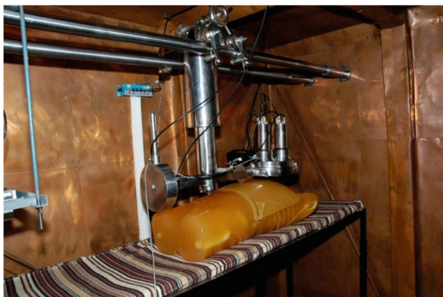
Fig. 10 Phoswich detector over JAERI phantom in standard lung measurement geometry
