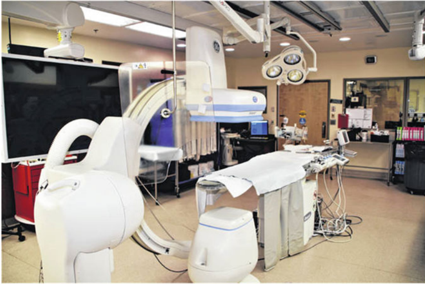
Fig. 10 Photograph of a C-arm fluoroscopy imaging equipment used for vascular and interventional procedures (Courtesy: Jupiter Hospital, Thane, Maharashtra, India)
