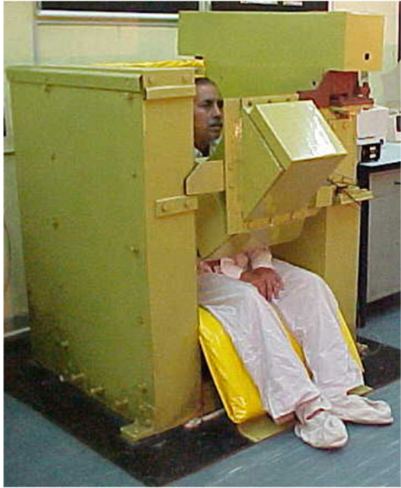
Fig. 8 Chair geometry used for whole body monitoring [3] (Courtesy: BARC Newsletter)
