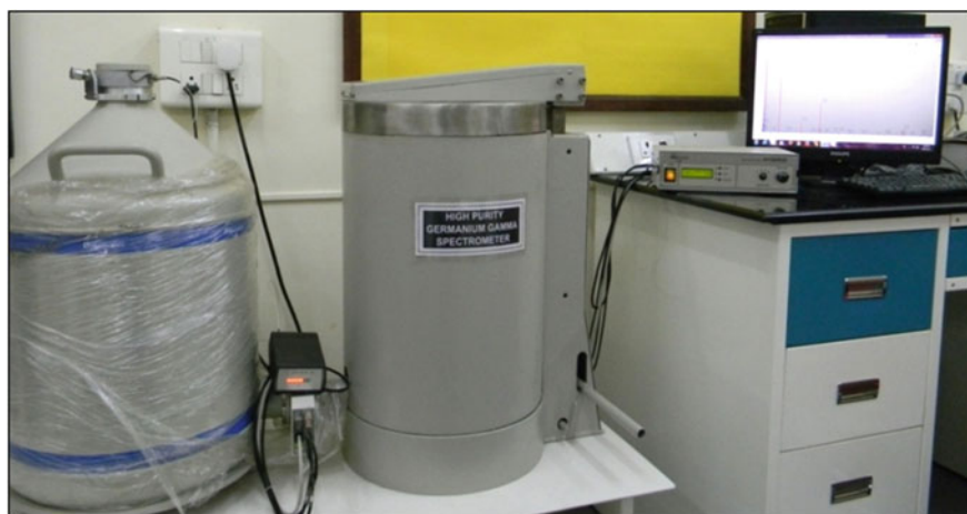
Fig. 16 HPGe gamma spectrometer for activity measurements of gamma emitting radionuclides
